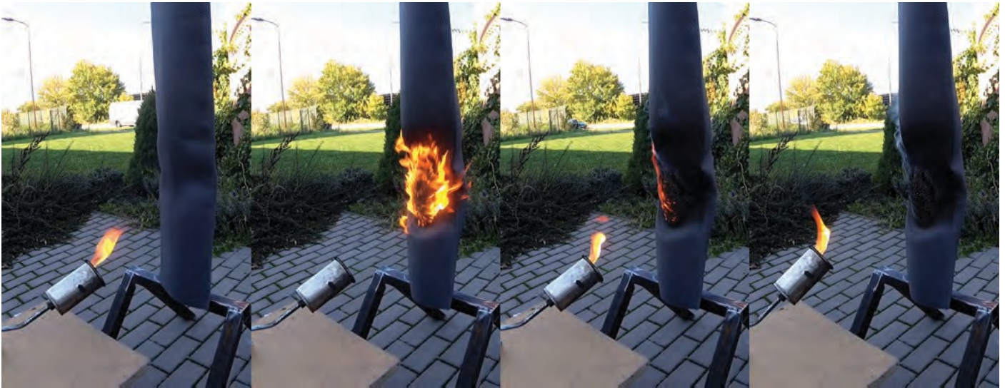
Testing the self-extinguishing properties of Nixus high pressure tubes
