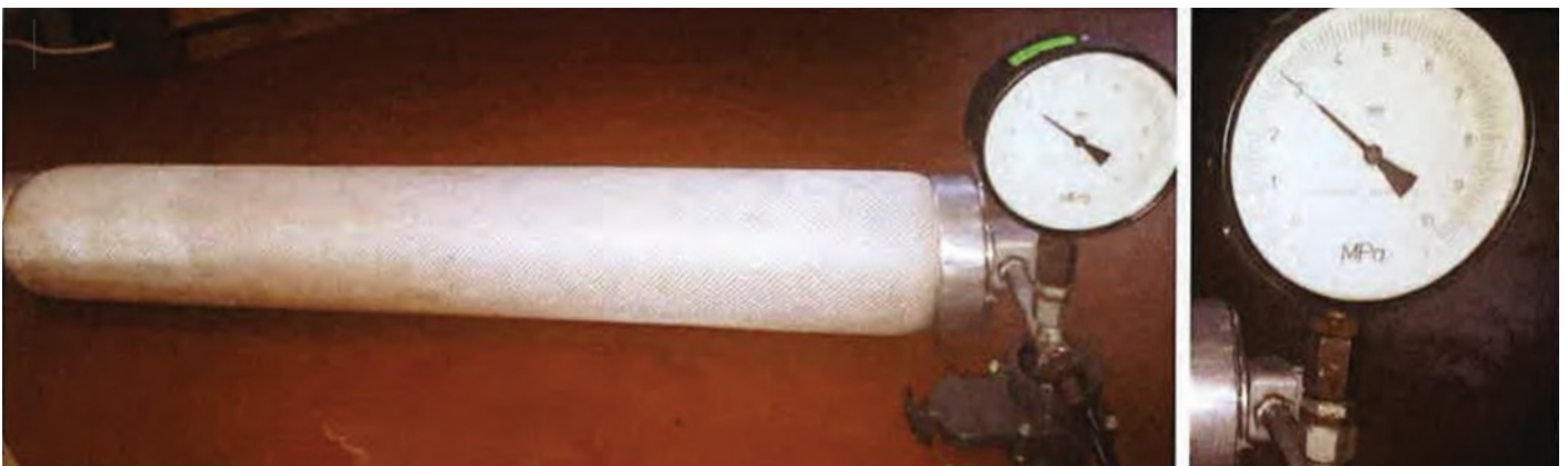
Pressure testing a beam to 30 bar
